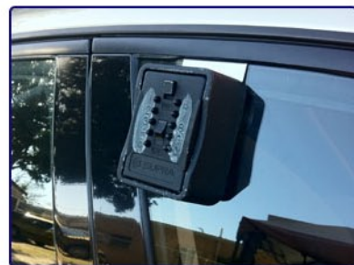
3 Access vehicle via key lock-box
